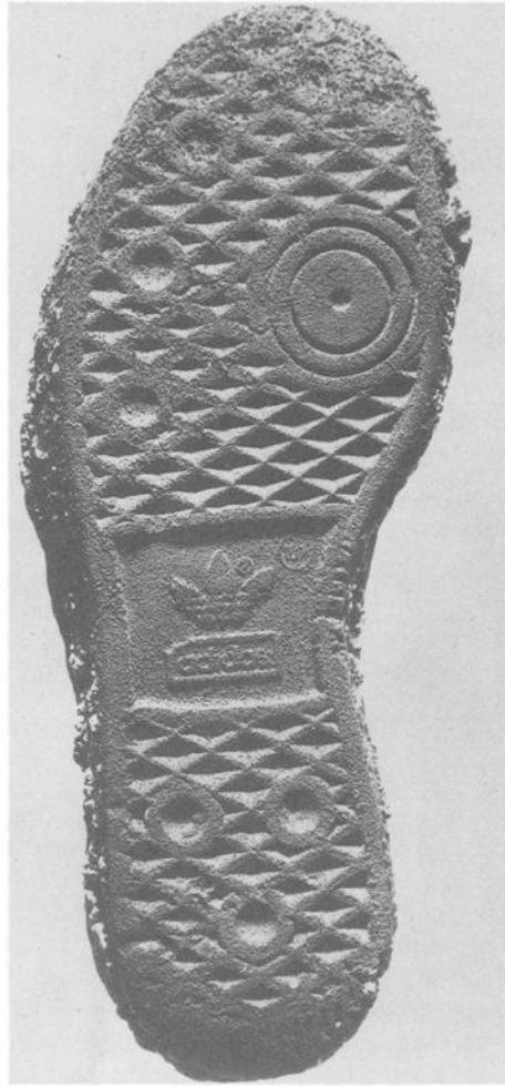
FIG. 5—Cast of the shoe impression in snow using Snow Print Wax.
