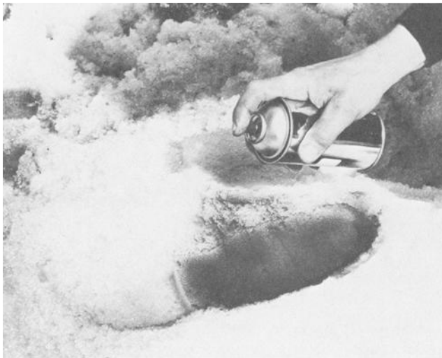
FIG. 1—Two or three thin layers of Snow Print Wax are sprayed into the impression.
