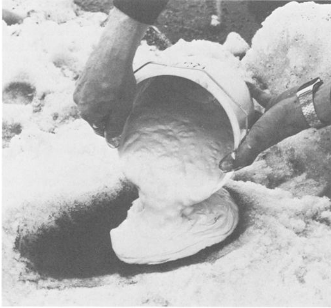
FIG. 2—A lukewarm (25°C) viscous mixture of plaster and water is poured into the layer of wax.
